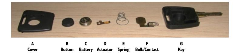
Insert part "F" into the hole on the key itself "G", so that the contact lays flat in the key. Place the spring on top of the contact, with the narrow end of the spring pointing up. Insert the actuator "D" in the key so that the lip on the lond end of the actuator is pointing up and laying against the bottom of the bulb. The round hole in the actuator will fit on a peg in the key "G".
